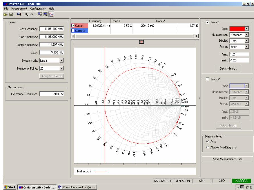
Place cursor 1 to the left most point of the trace, which corresponds to the Series Resonant frequency. The value of  $R_S$  is 10.56 Ohm with this measurement.
