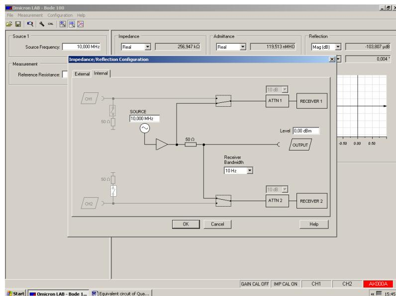
**3.)** Open the Calibration window and perform the impedance calibration by measuring “Open”, “Short” and “Load” as described in the Bode 100 user manual.
