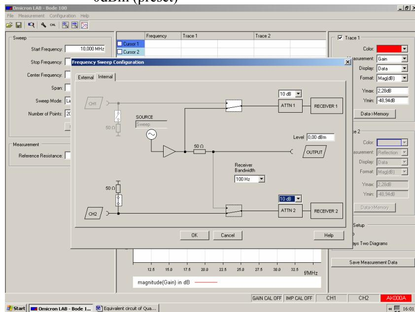
6.) Leave the configuration window by pressing OK and make following settings in the Frequency sweep window:
