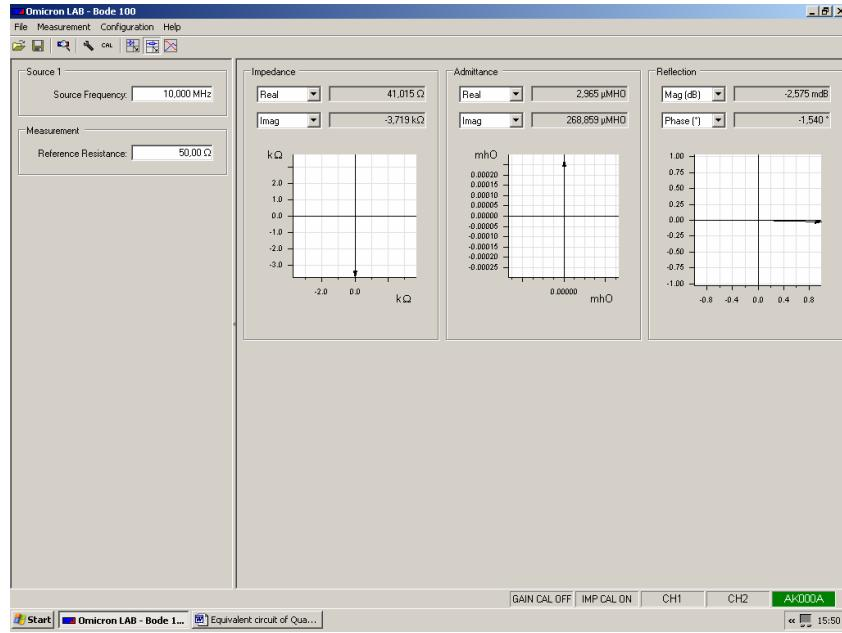
The readout for the Impedance is:  $Z = 41.015 - j 3719 \text{ Ohm}$  at 10MHz
