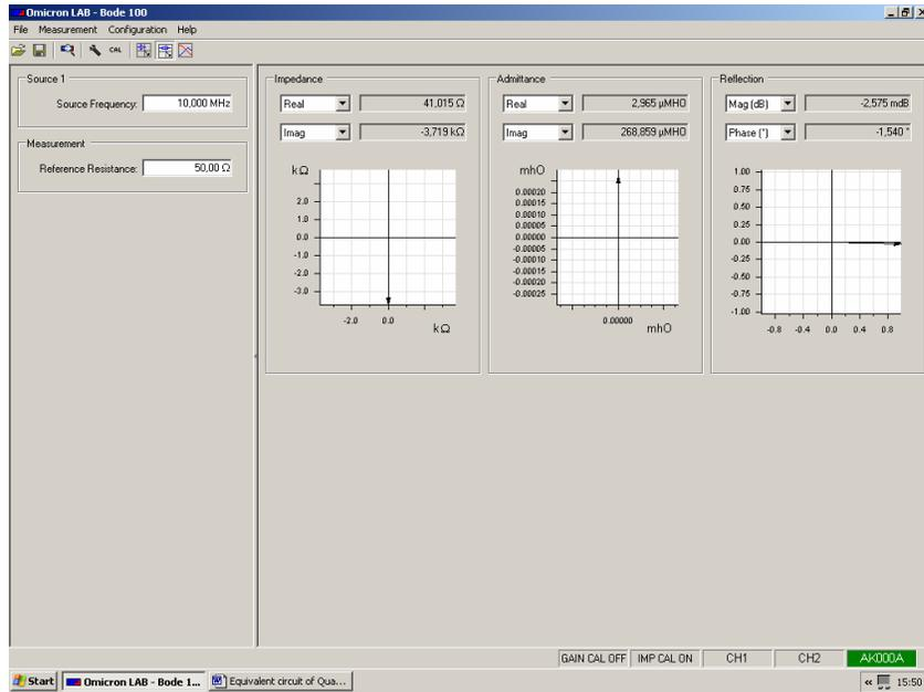
The readout for the Impedance is:  $\underline{Z} = 41.015 - j 3719 \text{ Ohm}$  at 10MHz
