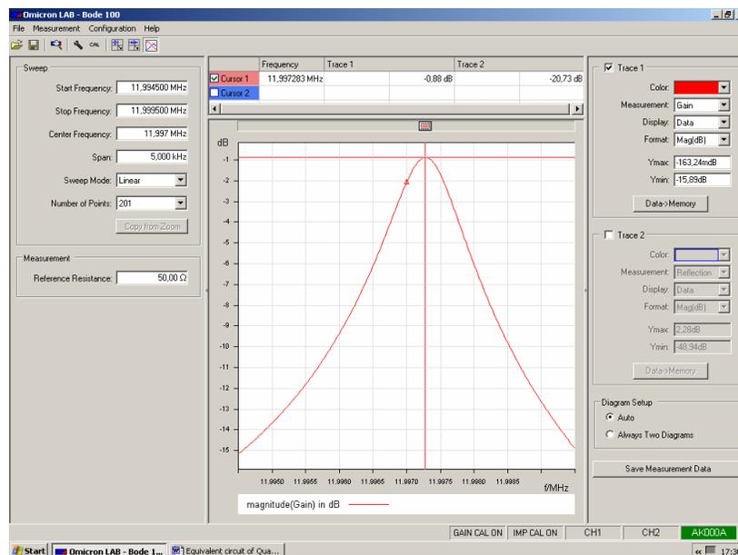
The readout of cursor 1 gives us an attenuation of 0.88dB. To calculate  $R_S$  we have to use the following equation:
