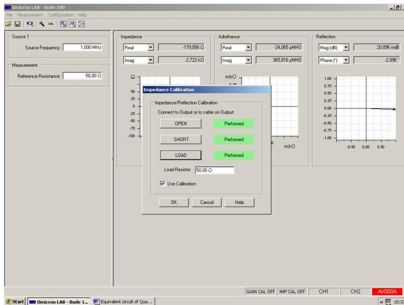
4.) Now we are ready to measure the Impedance of the crystal. Connect the measurement cable to the “IN” BNC connector and the “Short” to the “OUT” BNC connector of the Quartz filter on the Test PCB. By using right click and pressing “Optimize” in each diagramm you will get the following display:
